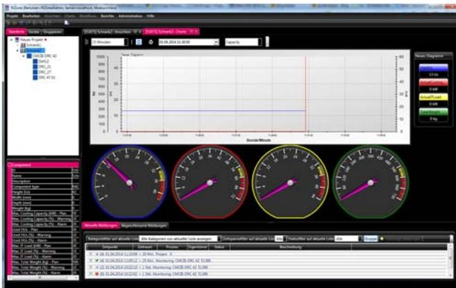
Capacity utilisation for height units, climate control, electrical power and weight. Data is represented in RiZone.
